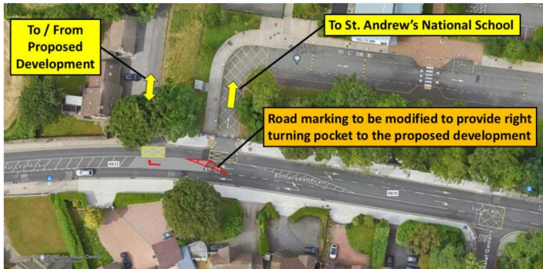
FIGURE 4.3 – PROVISION OF RIGHT TURNING POCKET AT WESTERN VEHICULAR ACCESS (SOURCE: GOOGLE MAPS, ANNOTATION BY EGIS)
