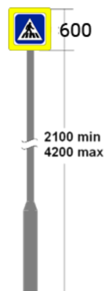
Figure 9.20A: Pedestrian Crossing Sign (for Pedestrian Crossings type RPC 001A)
