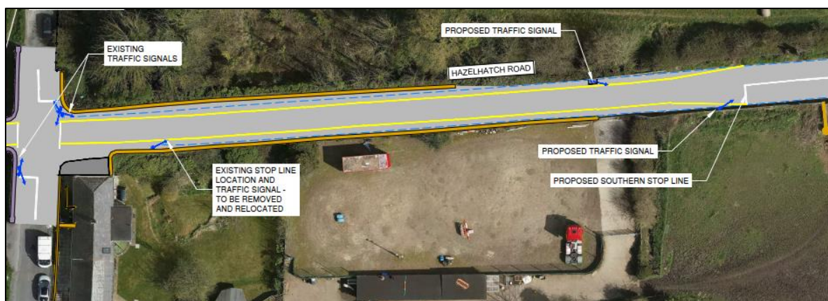
Figure 9: Preliminary design southern approach to bridge
