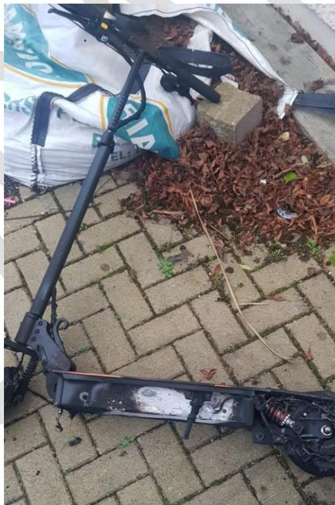
**Figure 15-2: Damage to e-scooter from battery fire**
