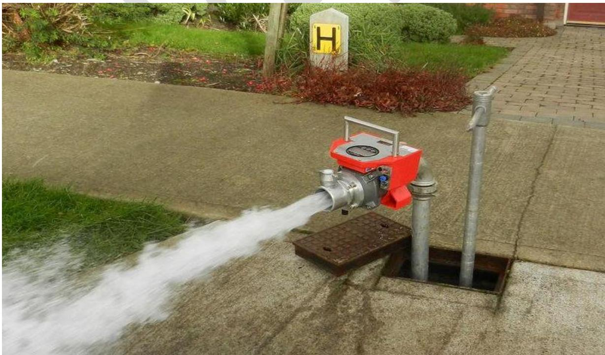
**Figure 9-1 Hydrant testing for pressure and flow-rate**
