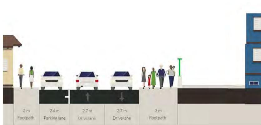
**Figure 6.51 - Route 7, Cross Section B-B Existing**
