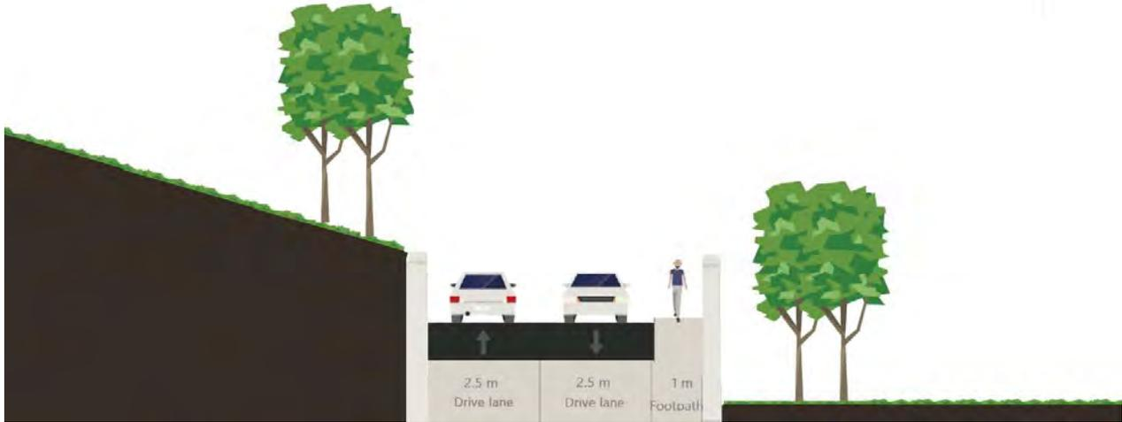
Figure 6.6 - Route 2, Cross Section B-B Existing
