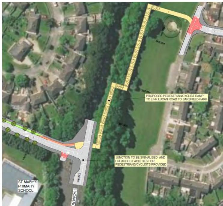
Figure 10.5 - Concept Design of Junction Layout and Ramp from Lucan Road to Sarsfield Park
