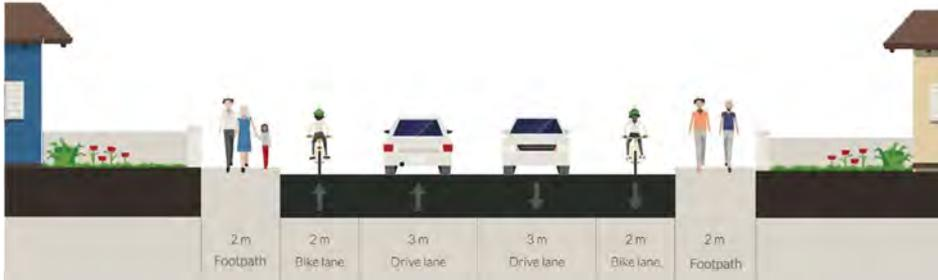
Figure 6.65 - Route 8C, Cross Section A-A Proposed
