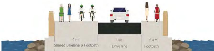
**Figure 8.15 - Route 11 B, Cross Section A-A Proposed**
