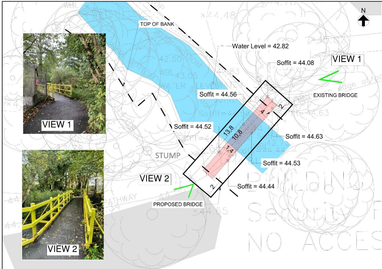
Figure 2-10: Plan View of Existing and Proposed River Griffeen Crossing No. 4 (Source: Arup)
