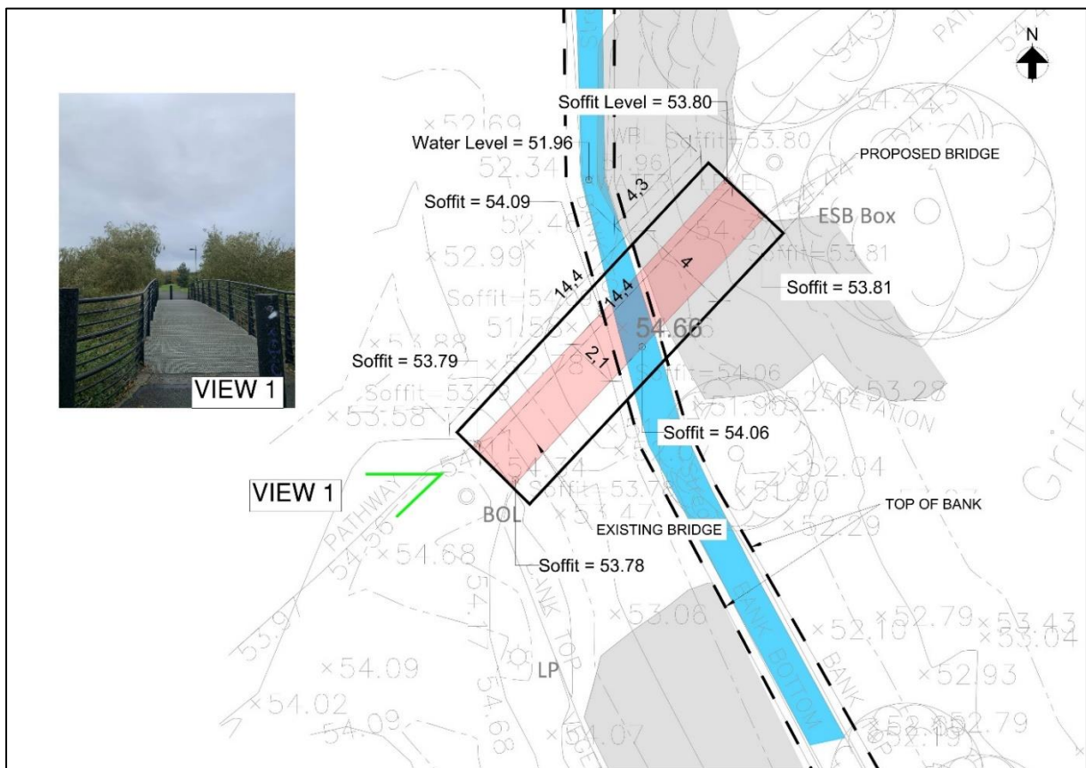
Figure 2-8: Plan View of Existing and Proposed River Griffeen Crossing No.2 (Source: Arup)
