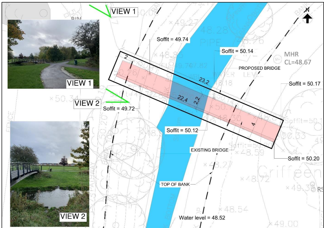
Figure 2-9: Plan View of Existing and Proposed River Griffeen Crossing No.3 (Source: Arup)
