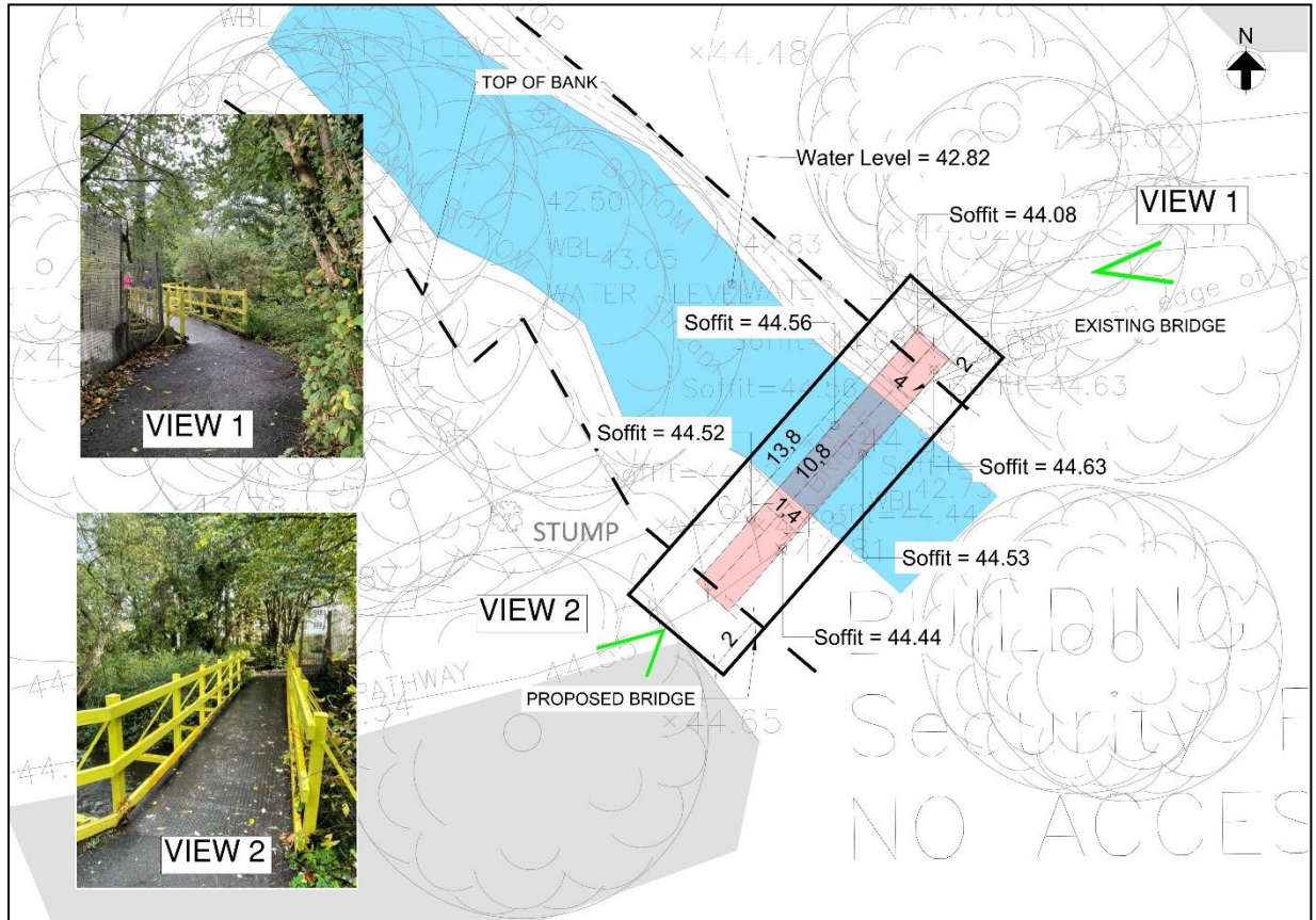
Figure 2-10: Plan View of Existing and Proposed River Griffeen Crossing No. 4 (Source image: Arup)
