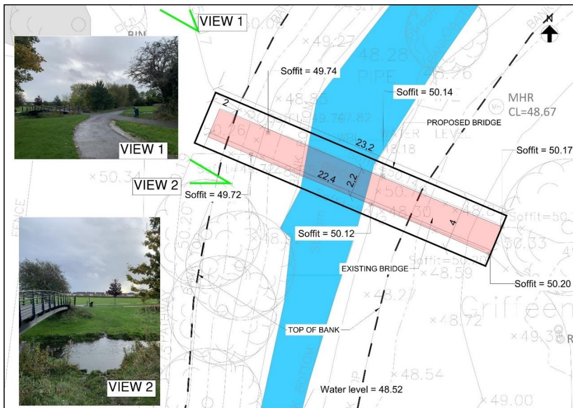
Figure 2-9: Plan View of Existing and Proposed River Griffeen Crossing No.3 (Source image: Arup)
