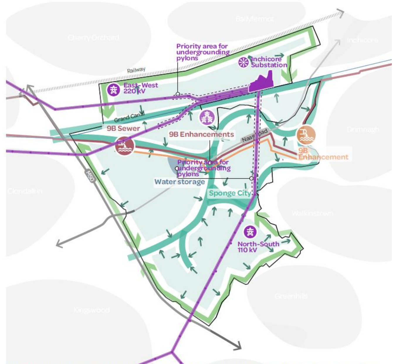
Figure 272. Overview of the potential utilities vision regarding energy, foul sewer and surface water drainage management strategies
