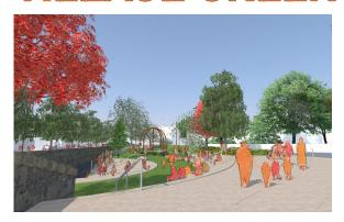
The works within the Green relate to improved footpaths, landscaping and a new bandstand structure capable of taking a temporary roof covering; the construction of new amphitheatre steps and seating providing access to the Griffeen river; the construction of a new seating area beside the Griffeen river facing Vesey weir and bridge. The existing metal guardrail will also be replaced.
