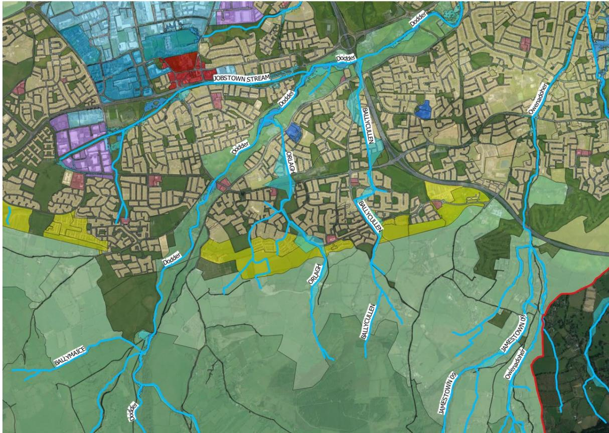
**Figure 2 Ballycullen Oldcourt - Flooding extents over laid on zoning maps**
