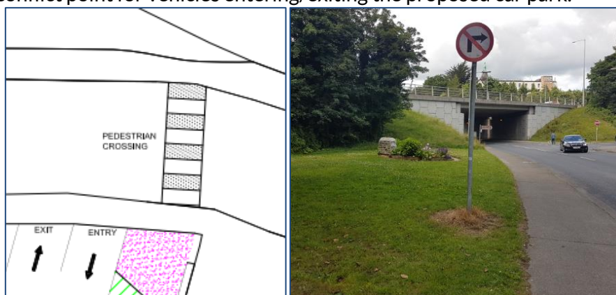
Figure 2-6: No right turn sign appearing to clash with location of proposed entrance/exit point to Site B
