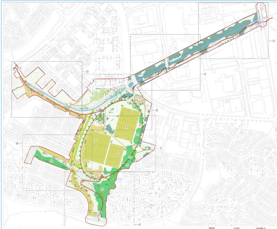
Figure 2-1 Proposed design layout of the upgrade to Killinarden Park and route of the Green Infrastructure Corridor. A larger version with a legend of this design is in Appendix A.
