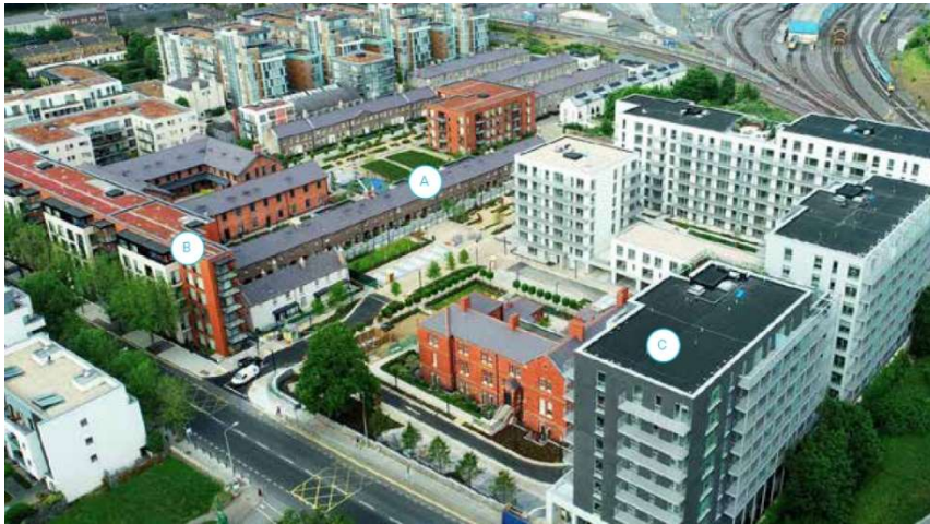
Contextual Heights at Clancy Quay Dublin - the 8-storey Building C can be expressed as a contextual height ratio of 4xCH relative to the historic buildings A or 1.25xCH relative to the newer development at Building B.
