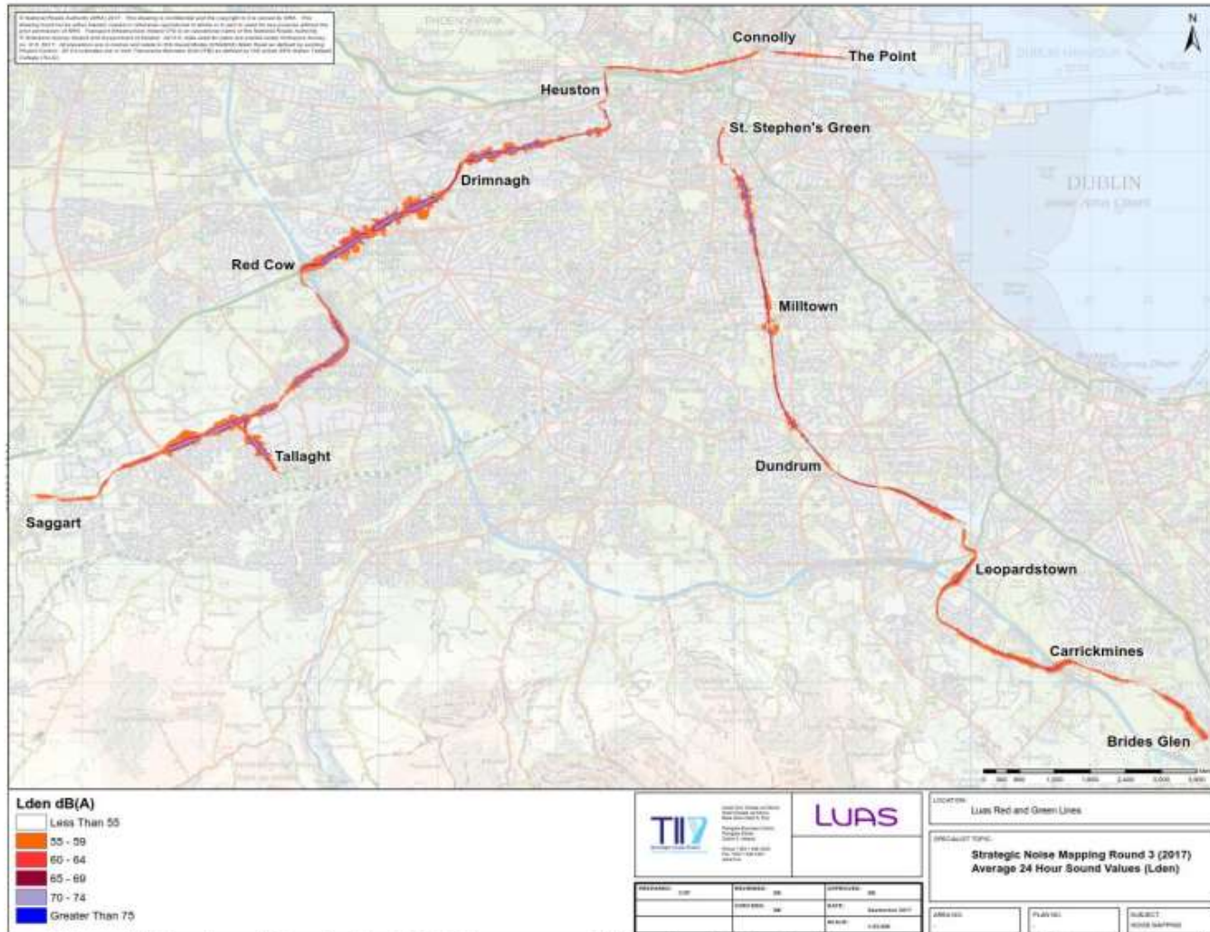
Figure 7: Lden Noise Level Bands for 2016 Assessment Year for Major Railways – Transport Infrastructure Ireland
