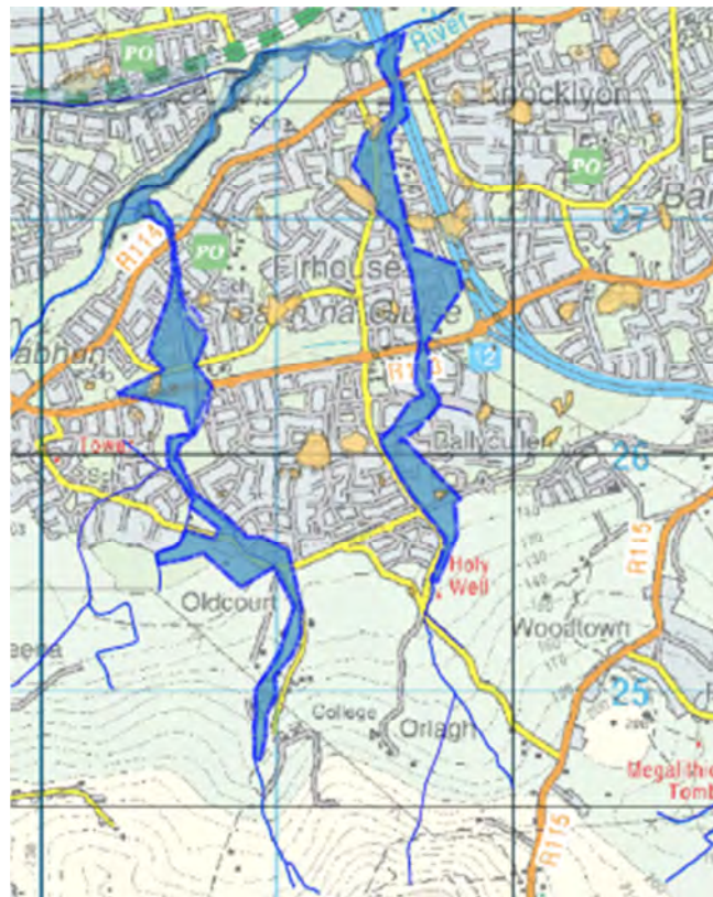
Figure 6.5 Indicative fluvial, pluvial flood zones and 2011 flood locations in Ballycullen & Oldcourt
