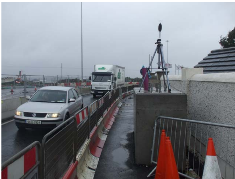
Picture 3: Shows the placement of the outdoor microphone during the daytime hours positioned 1.2m above the boundary wall to allow a free-field measurement to be conducted, minimising the effects of reflection from the boundary wall.
