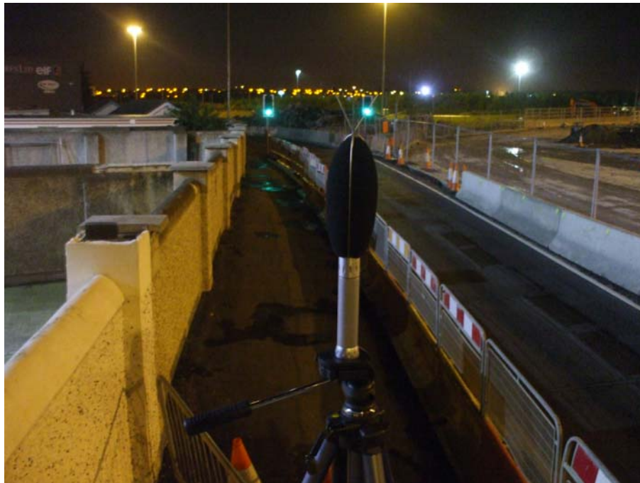
Picture 4: Shows the placement of the outdoor microphone during the night time hours positioned 1.2m above the boundary wall to allow a free-field measurement to be conducted, minimising the effects of reflection from the boundary wall.
