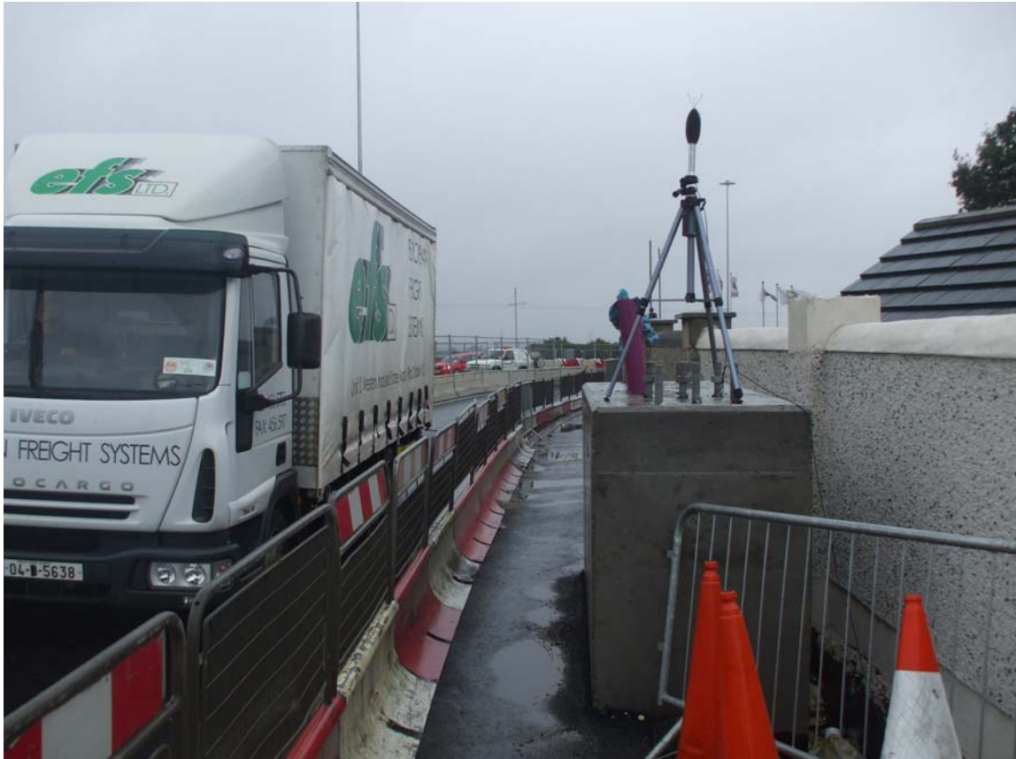
Picture 2: Noise measurements being conducted at the perimeter of the Traveller unit.
