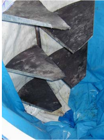
Figure 4.2 “Glance-Off” Plates in Danish Bring Banks
